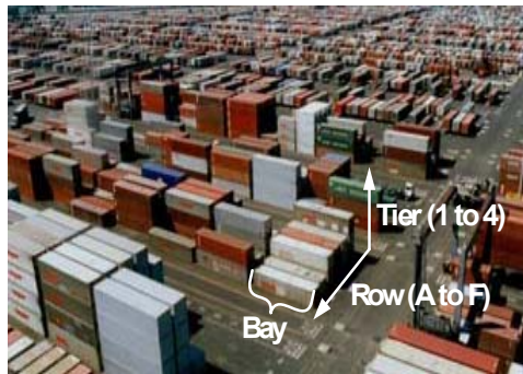
Figure 1 Illustration of bay, row, and tier in a yard block (see online version for colours)
