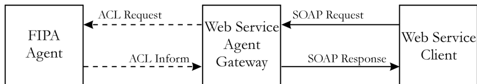
Fig. 3. The WSAG enables messages to flow between Web services and agents. ACL messages are exchanged asynchronously, whereas SOAP message exchange occurs synchronously. Copyright © 2002-2003 Agentcities Task Force (ACTF). All Rights Reserved.
