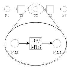
Figure 3. Refinement of P2 with a subnet
