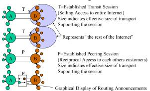
Finally, to demonstrate **traffic** going over the Peering or Transit pipe, we use directed lines as shown below. When the relevant traffic is destined to a specific network, the directed line is colored to represent traffic destined to the colored ISP. If traffic destination is not relevant, the color black is used. The thickness of the line represents the amount of traffic. Other variations will be presented as they arise during peering plays.
