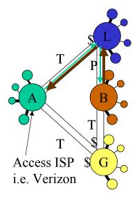
From my conversations I heard of two tactics to force traffic to go along the path that costs the target ISP the most money to access the access providers. The first technique is to simply stop announcing its routes to the target's Peer. This forces all traffic to use the alternative path, resulting in increased transit fees for the target ISP.
