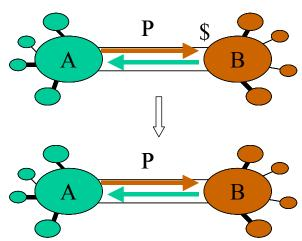
The router configurations, exchange point arrangements, and all peering interconnections logistics can proceed as if they were a free peering arrangement. When both parties agree the peering prerequisites are met, the settlement is no longer implemented and free peering is established.
