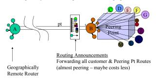
Note that only the routes announced *to* the partial transit provider at the exchange are propagated to the customer. While this is not "Peering" by my definition, it is a useful tactic to quickly obtain exchange point routes and it can be very inexpensive 40 for the Partial Transit provider to provide.
